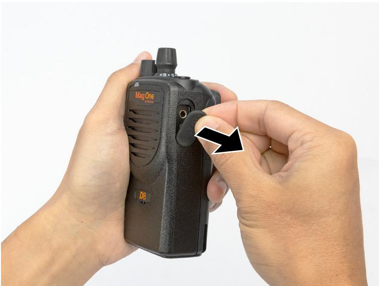
**Postrequisites:** Replace the dust cover when the universal connector is not in use.
