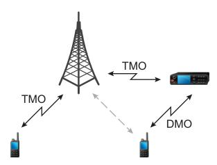
Radio behavior when radio detects a potential repeater signal or connects to a gateway:
