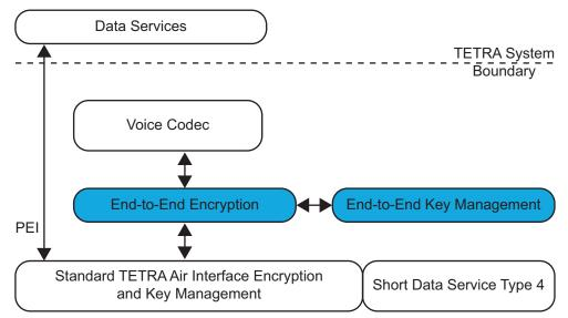
The End-to-End Encryption (E2EE) feature resolves this issue by encrypting the voice information before it is packed into the PDU. This message is also encrypted according to the over-the-air encryption of the TETRA standard. Thus, when the Base Station decrypts the PDU containing voice information, the voice part remains protected by encryption until the called radio receives the voice and decrypts it.
