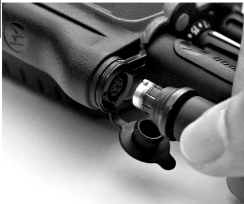
Figure 1. To insert the accessory, hold (as shown in Figure 1) the end with the connector, align with audio adapter attached to radio, and push.
