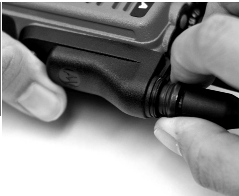
Figure 2. To remove the accessory, hold (as shown in Figure 2) firmly and pull.
