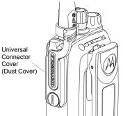
Place the universal connector cover loop over the attached antenna. Slide it all the way down to the base of the antenna.
