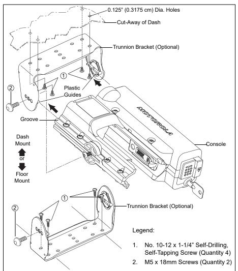
Figure 2: Console Installation Detail
