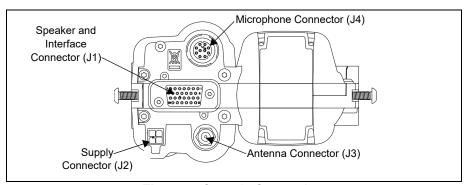
Figure 7: Console Connections
