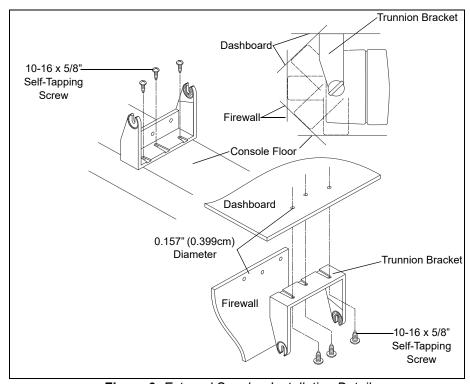
Figure 9: External Speaker Installation Detail
