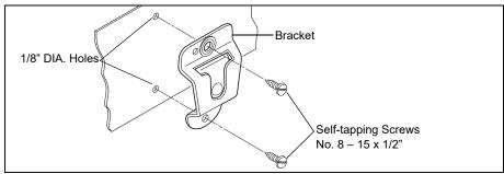
Figure 3: Microphone Bracket Installation Detail
