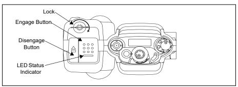
Figure 13: APX VA Mechanisms for Radio Installation/Extraction
