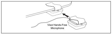
Figure 4: Visor Microphone Installation Detail
