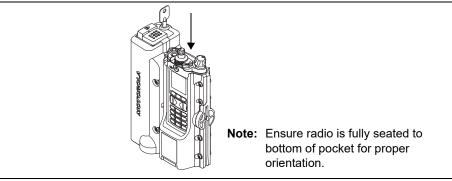
Figure 12: Radio Installation into APX VA Unit
