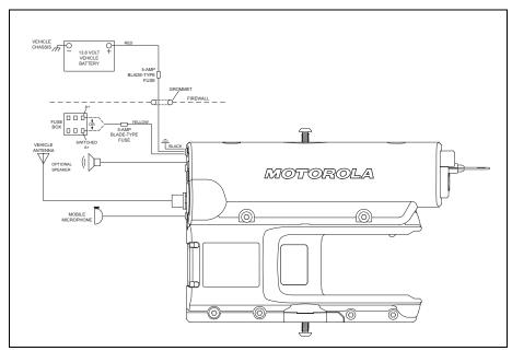
Figure 8: Console Cabling
