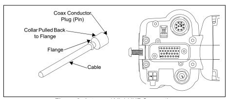
Figure 6: Antenna / Mini-UHF Connection
