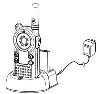
The drop-in charger will also sequentially charge a spare Li-Ion battery. The spare battery will not begin to charge until the radio battery is fully charged. Both batteries will charge in approximately 8 to 10 hours.
