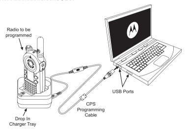
To program, connect the CLS Series radio via the Drop-in Charger Tray and CPS Programming Cable to your computer as shown in the picture above. Prior to programming, verify that the switch in the Programming Cable is in the 'Analog(\*\*)' position.
