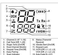
Note: The radio screen will dim 5 seconds after the last button is pressed. Radio screen will turn off after another 5 seconds for battery saving purpose, only an LED will be shown blinking.
