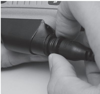
Figure 2. To remove the accessory, hold connector top firmly and pull.
