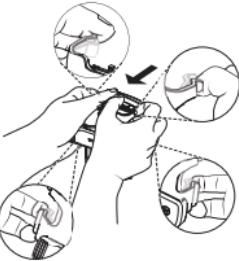
3. Ensure the bottom tabs are engaged with the housing and press the battery cover towards the pager until it clicks into place.
