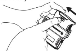
3. To remove the battery cover, pull the latches on both sides to disengage the battery cover from the pager.
