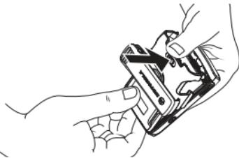
4. Lock the battery cover by sliding the latch button to the right.
