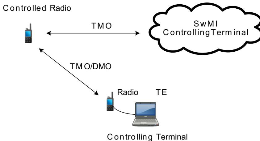
The SDS remote control functionality works in both Trunked Mode Operation (TMO) and Direct Mode Operation (DMO) and the remote control PDUs are sent using Terminal Equipment (TE).
