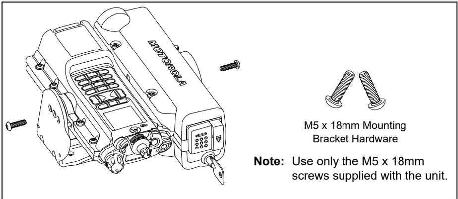
*Figure 1: Console Installation Detail*
