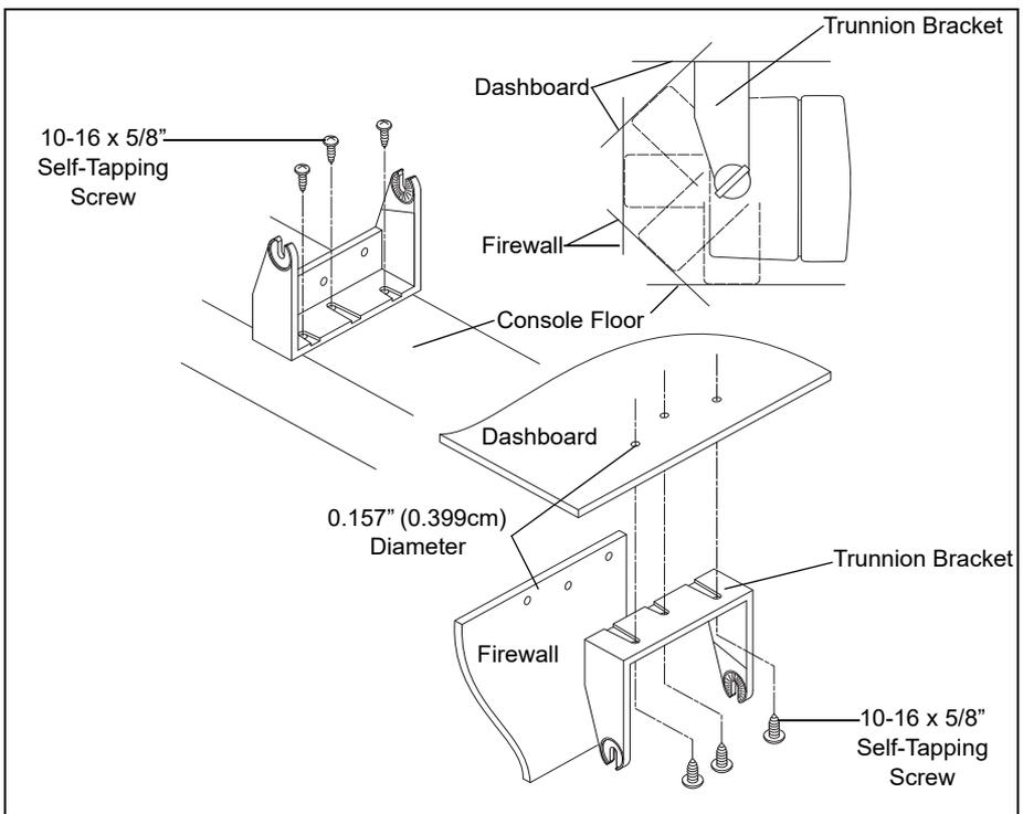
**Figure 9: External Speaker Installation Detail**
