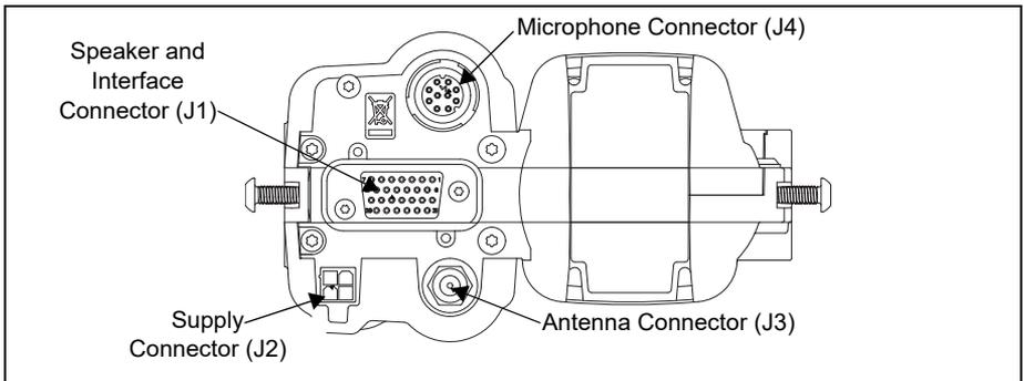
**Figure 7: Console Connections**
