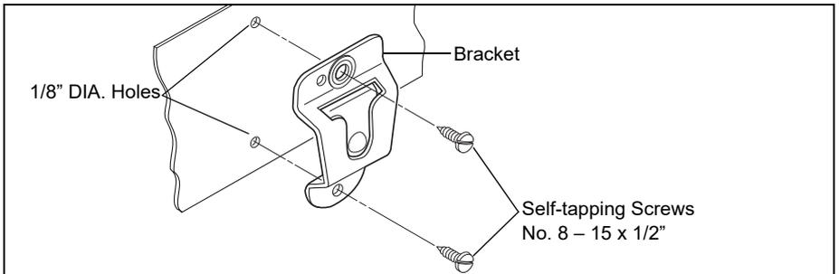
**Figure 3: Microphone Bracket Installation Detail**
