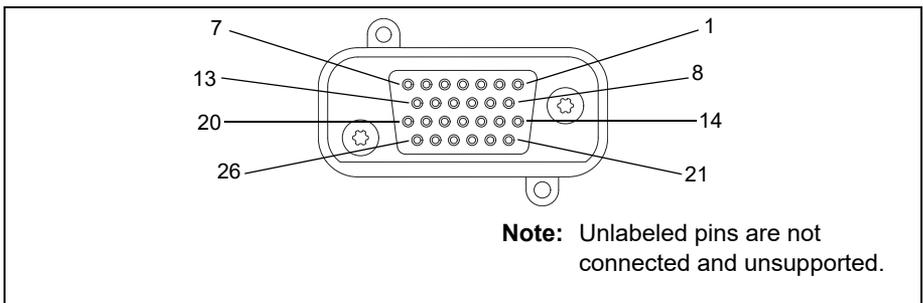
**Figure 10: J1 Connector Definition**
