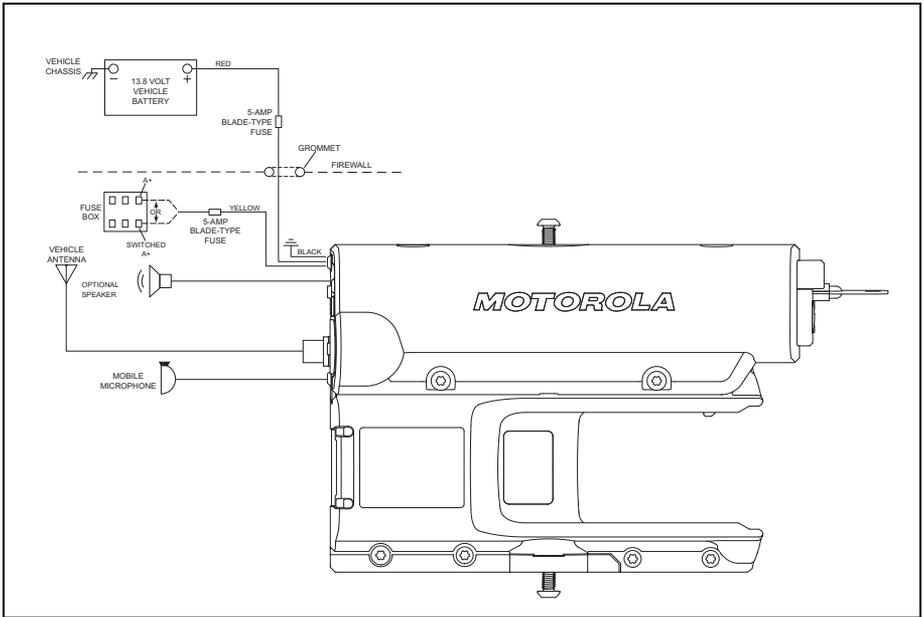
**Figure 8: Console Cabling**
