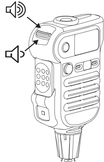
**NOTE:** A single press of the volume switch increases or decreases the volume by one step.
