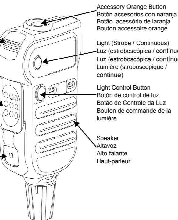
**WARNING:** Use the RSM in an upright position for proper water drainage.
