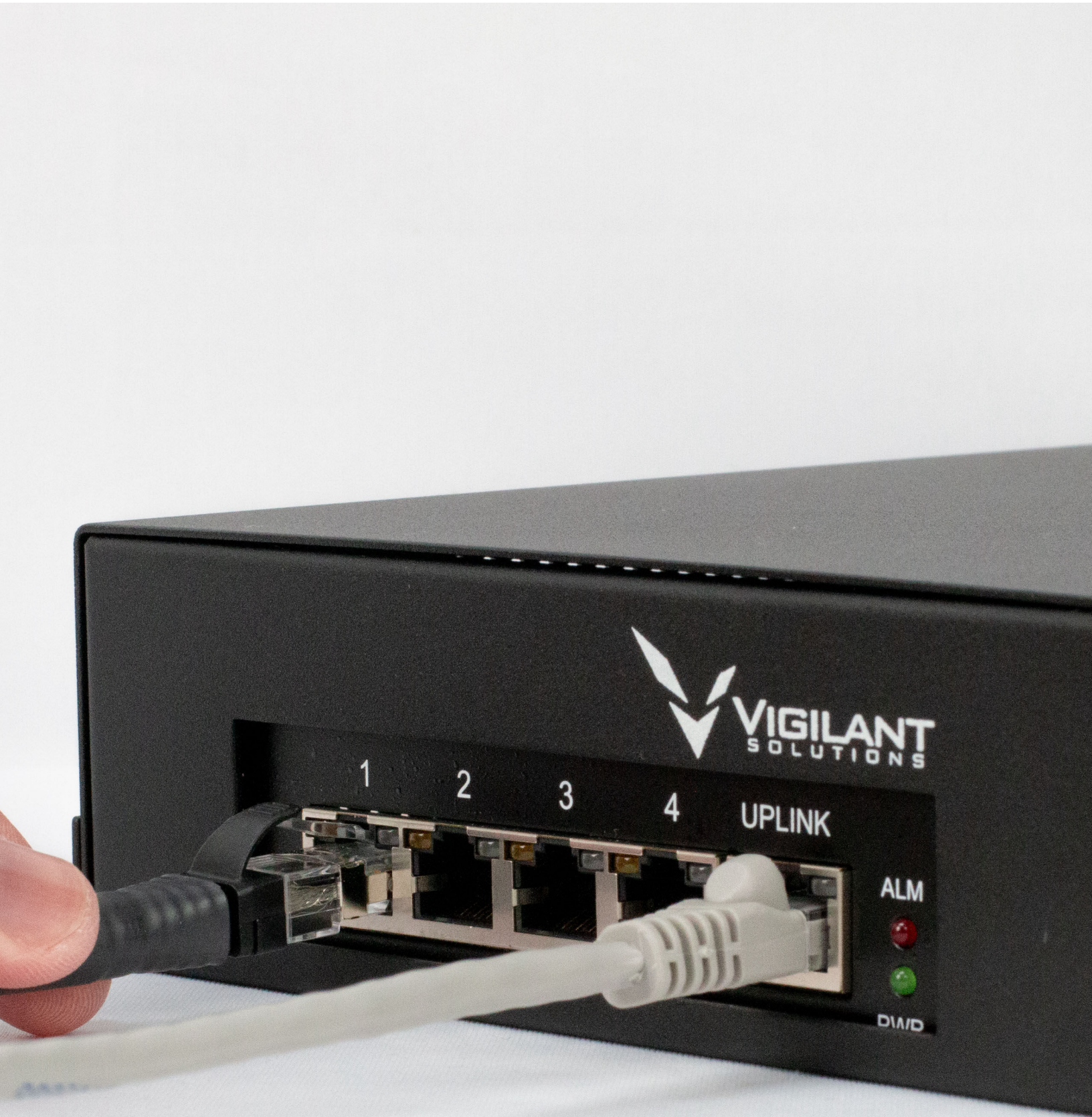
Figure 8: Camera Cable to PoE Injector
