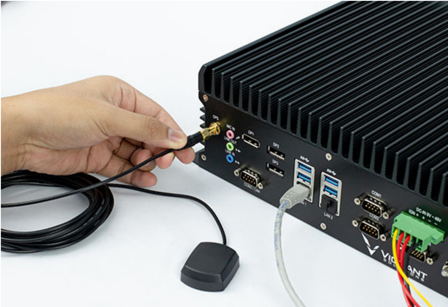
Figure 5: GPS Cable to VLP Processor
