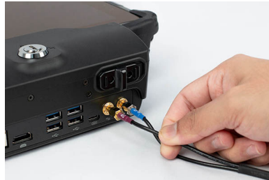
Figure 10: 4G Connector to VLS Tablet Docking Station
