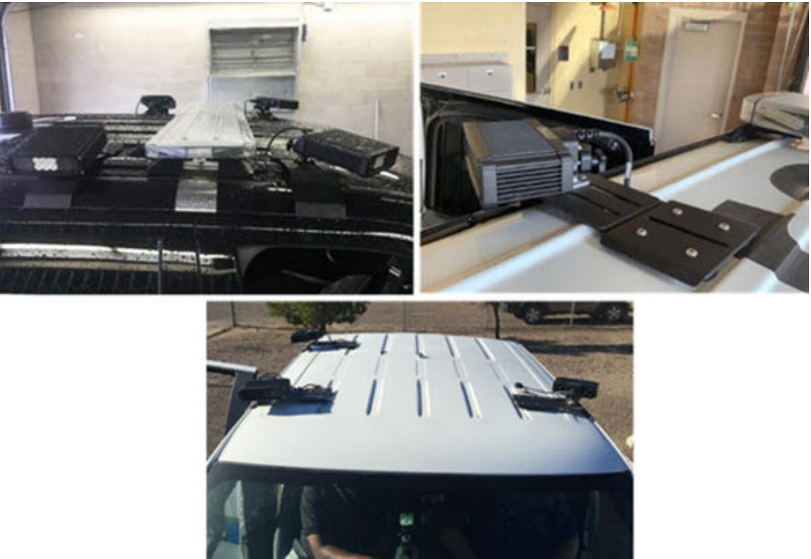
Lip mount brackets secure to the trunk lip using magnet feet and tension screws on the lip.
