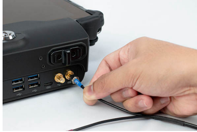
Figure 33: 4G Connector to VLS Tablet Docking Station
