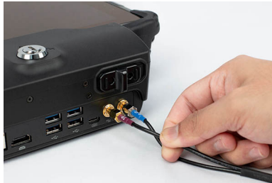
Figure 33: 4G Connector to VLS Tablet Docking Station
