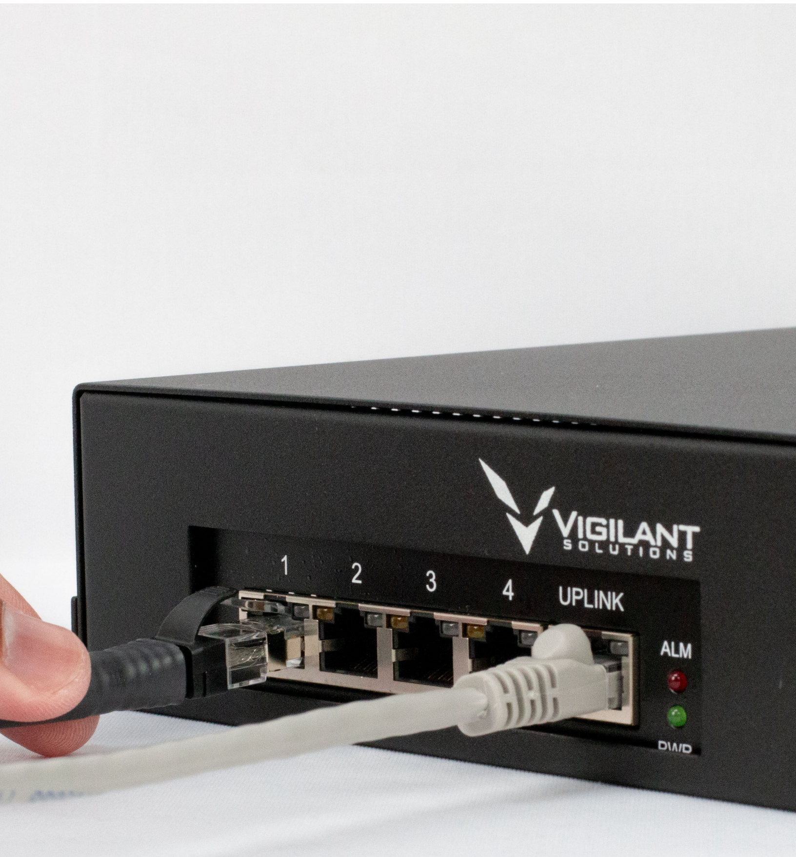
Figure 31: Camera Cable to PoE Injector
