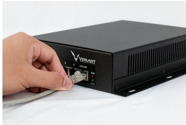
Figure 30: Ethernet Cable to PoE Injector
