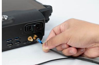
Figure 10: 4G Connector to VLS Tablet Docking Station
