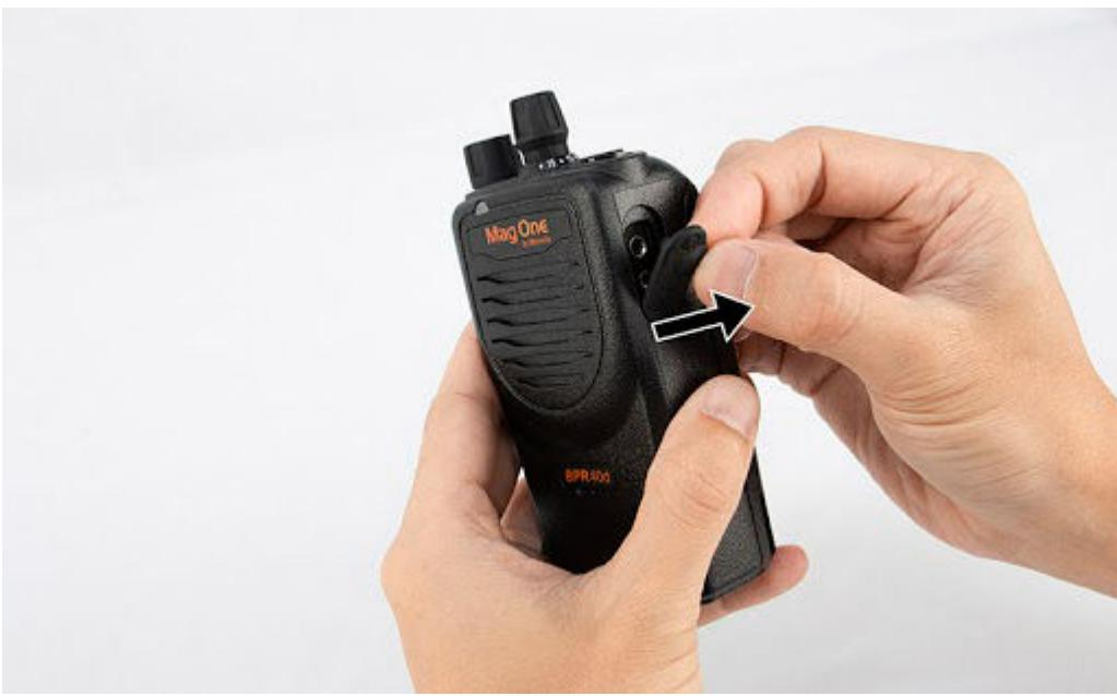
**Postrequisites:** Replace the dust cover when the universal connector is not in use.
