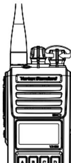
2. To turn off the radio, turn the **Volume/Power** knob counterclockwise.
