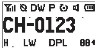
The PL or DPL icon appears on the screen. If **DPL** is displayed, DCS system is activated. If **PL** is displayed, CTCSS system is activated.
