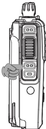
2. To switch to lower power to prolong the battery life, short press the **Side-2** button.
