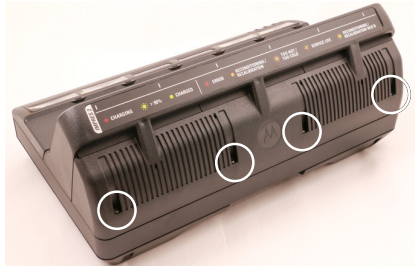
Figure 32: Shroud Screws Installation
