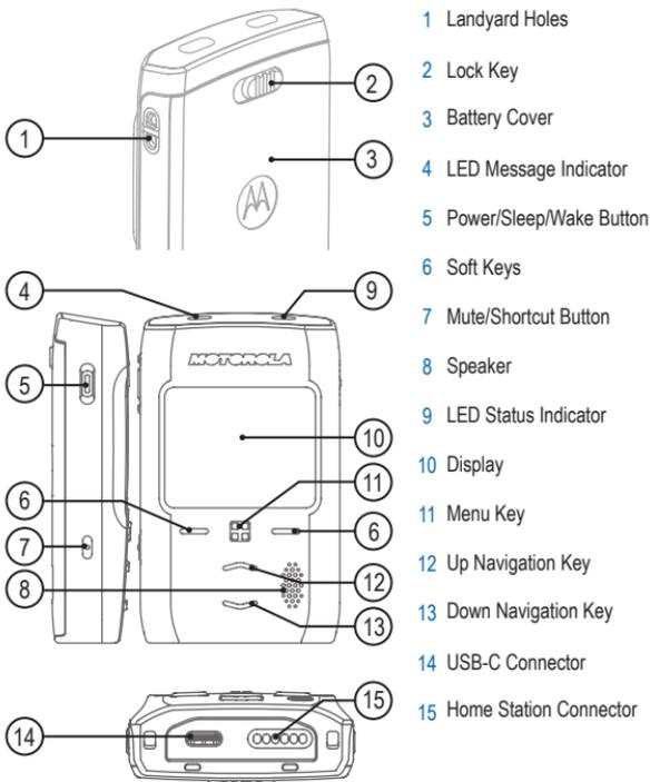
\* The LED indication and flashing pattern can be configured in the Customer Programming Software (CPS).
