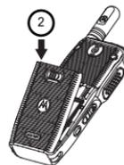
2. Insert the bottom tabs of the battery cover into the slot. Press down the top part followed by the middle part of the battery cover.
