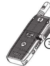
3. Slide the latch into lock position.
