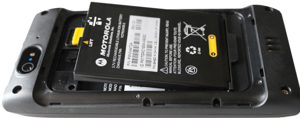
Figure 7: Installing the Battery
