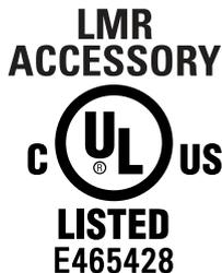
LMR Accessory for use in HAZ.LOC. Are listed by UL to non-incendive standards: UL121201 and CAN/CSA C22.2 No. 213-17 as safe for use in Class I, Division 2, Group A,B,C,D; Class II, Division 2, Group F,G; Class III, T3C. Tamb = -20°C to +60°C.
