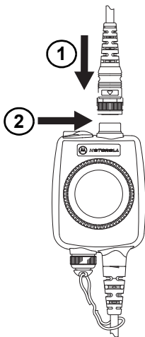
Figure 3. Location to Attach Bone Conduction Ear Microphone to Interface Module
