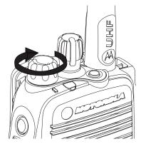
To turn off the radio, rotate this knob counterclockwise until you hear a click
