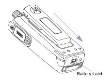
To remove the battery, turn the radio off. Move the battery latch into unlock position and hold, and slide the battery down and off the rails.
