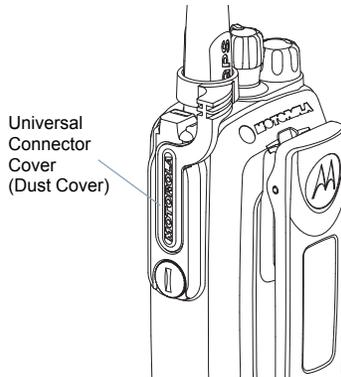
Place the universal connector cover loop over the attached antenna. Slide it all the way down to the base of the antenna.
