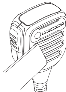
Figure 2: Vacuum speaker grill and mic ports. Do not cover all openings at once.
