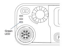
**NOTE:** The green LED lights up while the radio is transmitting and blinks rapidly when the radio is receiving a privacyenabled call.
