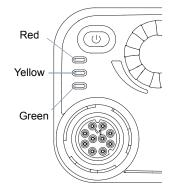
**Double blinking yellow** – Radio is no longer connected to the repeater while in Capacity Plus or Linked Capacity Plus, all Capacity Plus channels or Linked Capacity Plus channels are currently busy.
