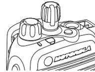
*To remove the antenna, turn the antenna counterclockwise. Make sure you turn off the radio and remove the universal connector cover (dust cover) first.*
