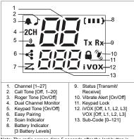
Note: The radio screen dims 5 seconds after the last button is pressed. LED blinks and the radio screen turns off after another 5 seconds for battery saving purposes. Press any button (except Flashlight button) to resume the display.
