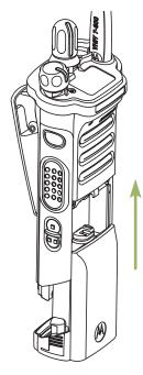
**2** To remove the battery, turn the radio off. Squeeze the release latches (A) at the bottom of the battery until the battery releases from the radio and remove the battery from the radio.
