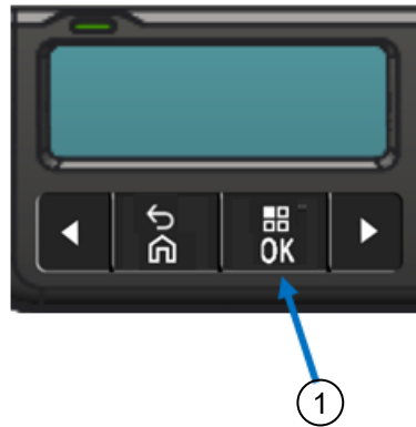
Figure 14: Menu Display Button for Entry to Analyzer Mode
