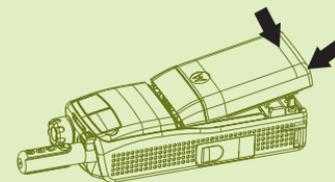
Remove the battery from its protective white paper box. Insert the battery top into the compartment as illustrated. Carefully press the battery bottom downward until it clicks into place.
