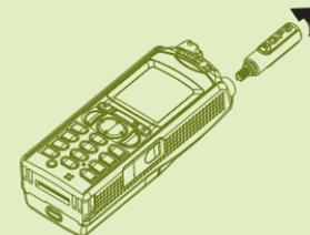
Turn the terminal off before attaching the antenna. Align the bottom of the antenna and the screw-in base on the top of the terminal. Turn clockwise until snug. Do not force.
