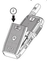
3 Slide the battery latch into lock position.
