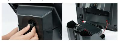
3 Slide the red battery lead onto the red terminal.
