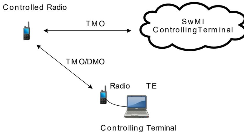
The SDS remote control functionality works in both TMO and DMO and the remote control PDUs are sent using terminal equipment (TE).
