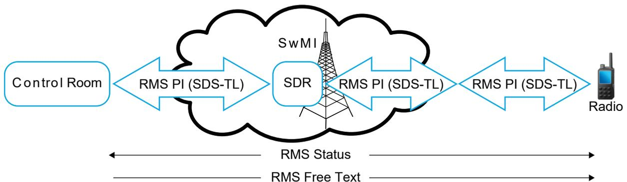
A Short Data Router (SDR) provides TETRA short data services between host applications connected to Dimetra Mobile Stations or between a host application connected to a Dimetra Mobile Station and a host application connected through the Dimetra Master Site. Furthermore the SDR provides TETRA short data services directly between two Dimetra Mobile Stations or directly between a Dimetra Mobile Station and a host application connected through the Dimetra Master Site.
