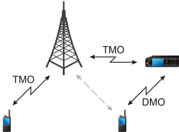
When the radio connects to a gateway, it plays a tone, displays the **Gateway available** message and shows an appropriate icon. When the radio loses connection with the gateway, it plays a tone, displays the **Gateway not available** message, and the gateway icon is blinking. Messages and sounds are configured by the service provider.
