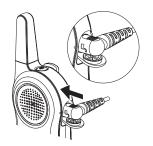
2. Rotate the audio jack connector 90 degrees upwards to lock.
