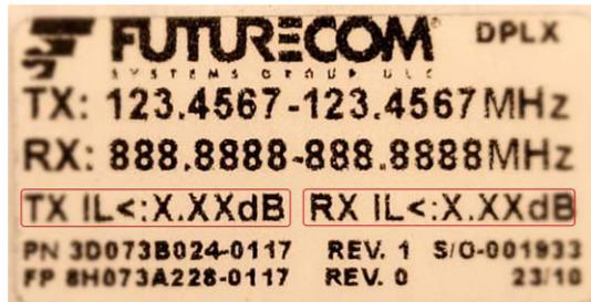
For Duplexers from different manufacturers, refer to the manufacturer's specification for Duplexer losses and enter the values into the FRC **Duplexer Losses** fields. You can create different **Deployment Profiles** for each duplexer (if multiple Duplexers are being used) by selecting the appropriate Deployment Profile when inserting a different Duplexer. See the *PDR8000 Portable Digital Repeater Programming Guide* for more information.
