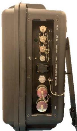
When operating open-case, the PDR8000 is to be placed flat on its large surface. Open case operation provides the best cooling capability.
