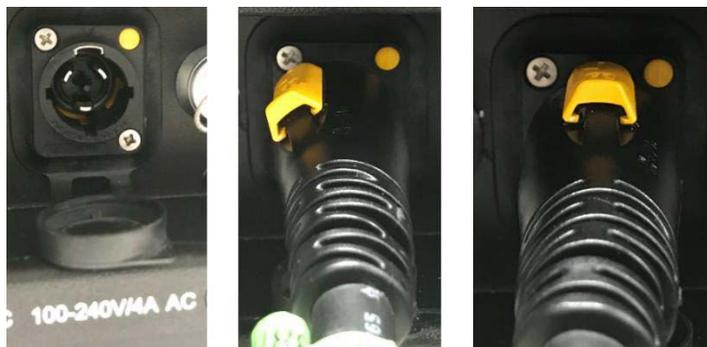
4. Connect the other end of the AC power cable to the AC power supply.
