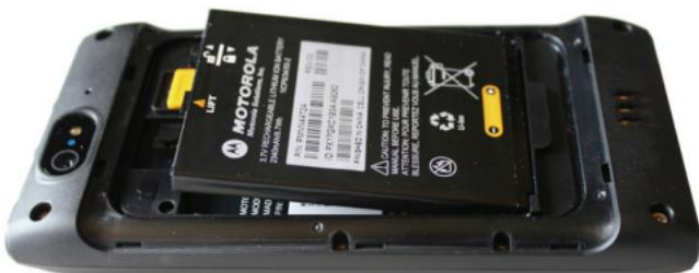
3. Press the top of battery into place.
