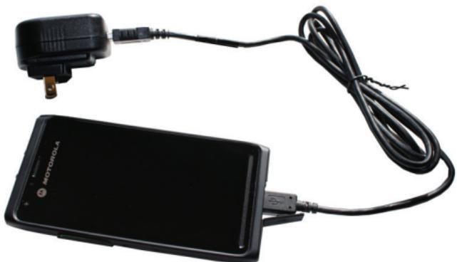
5. The charge and notification LED turns solid red, indicating the battery is charging. When the battery is fully charged, the LED turns solid green.
