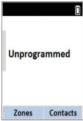
The image shows a screenshot of the radio's display during the initial activation process. It displays the text "Unprogrammed" in the center. At the bottom, there are two tabs: "Zones" and "Contacts".             | <b>LED :</b><br>-<br><br><b>Tone :</b><br>Continuous Unprogrammed | Radio is in the unprogrammed state.                             |
