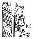
Figure 5: Attaching the Accessory Connector to Non-keypad Radio
