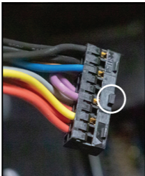
Figure 6: The connector is keyed and only fits one way into the charger.
