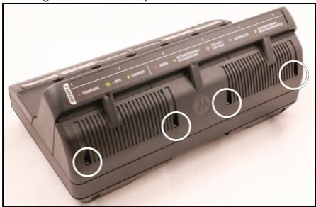
Figure 1: The four screws on the rear shroud.
