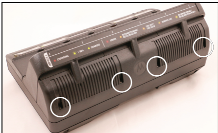
Figure 13: Shroud screws installation.
