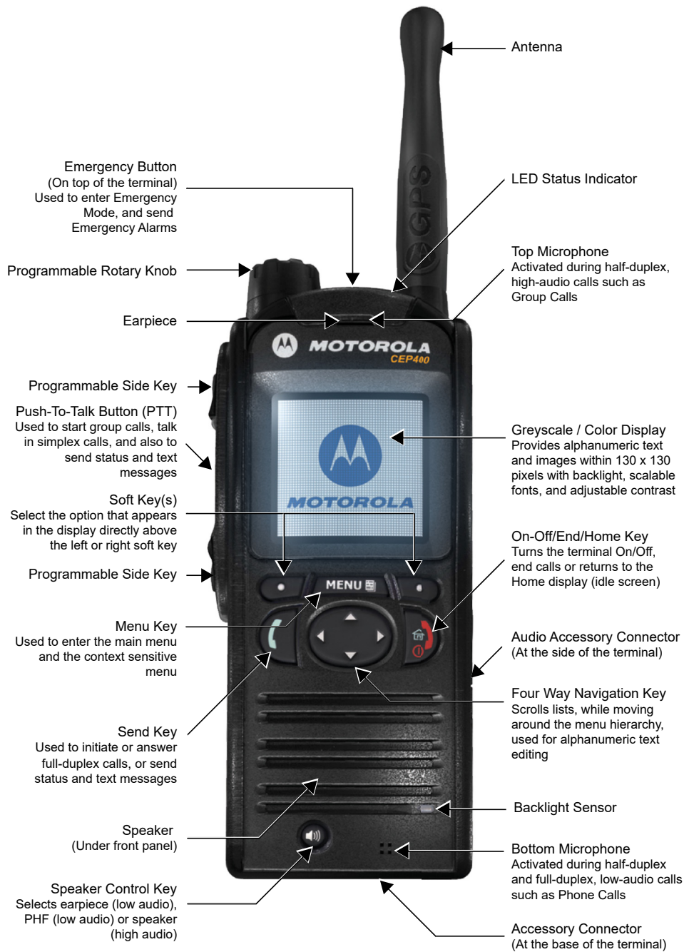
Figure 3-6 CEP400/MTP830 Portable Terminals Controls and Indicators
