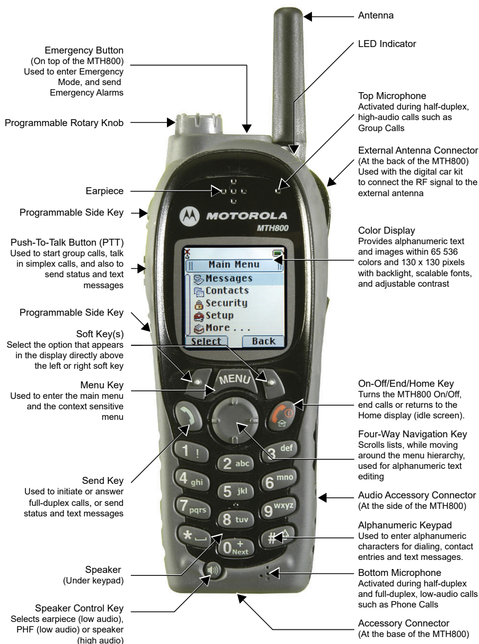
Figure 3-1 MTH800 Portable Terminal Controls and Indicators
