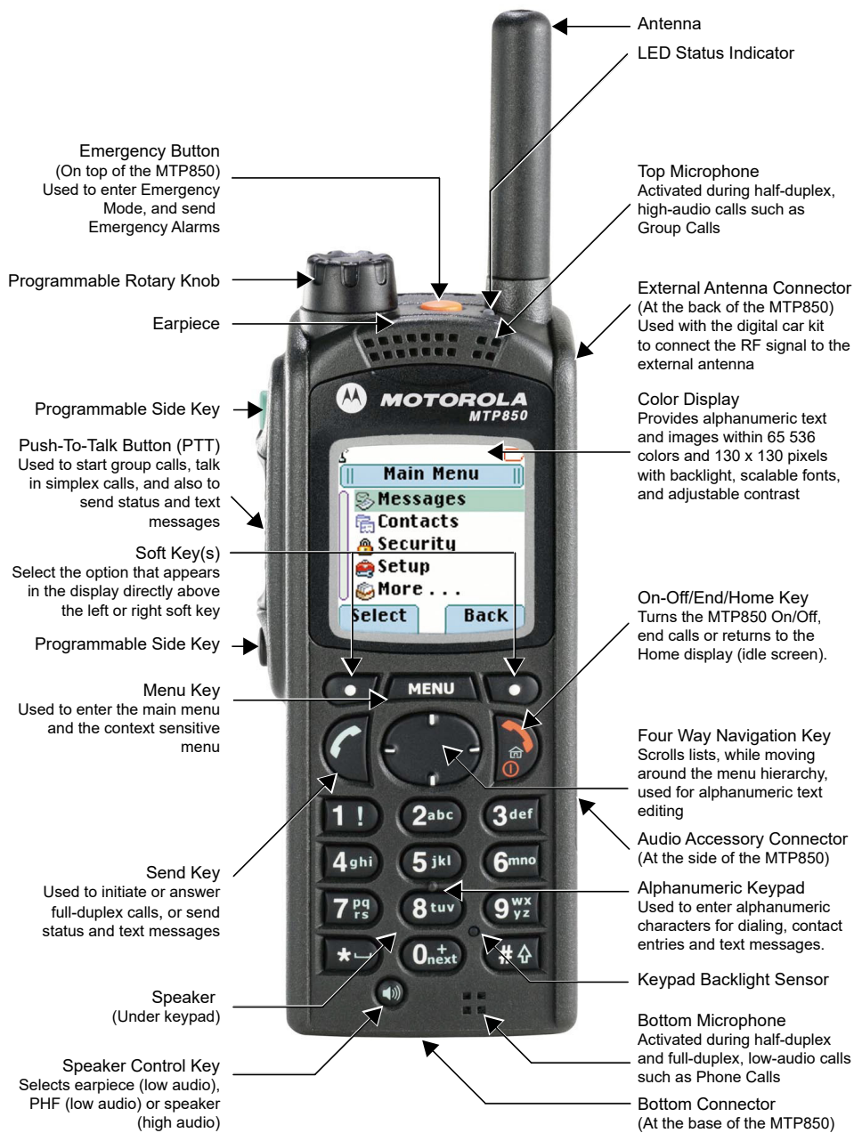
Figure 3-2 MTP850 Portable Terminal Controls and Indicators
