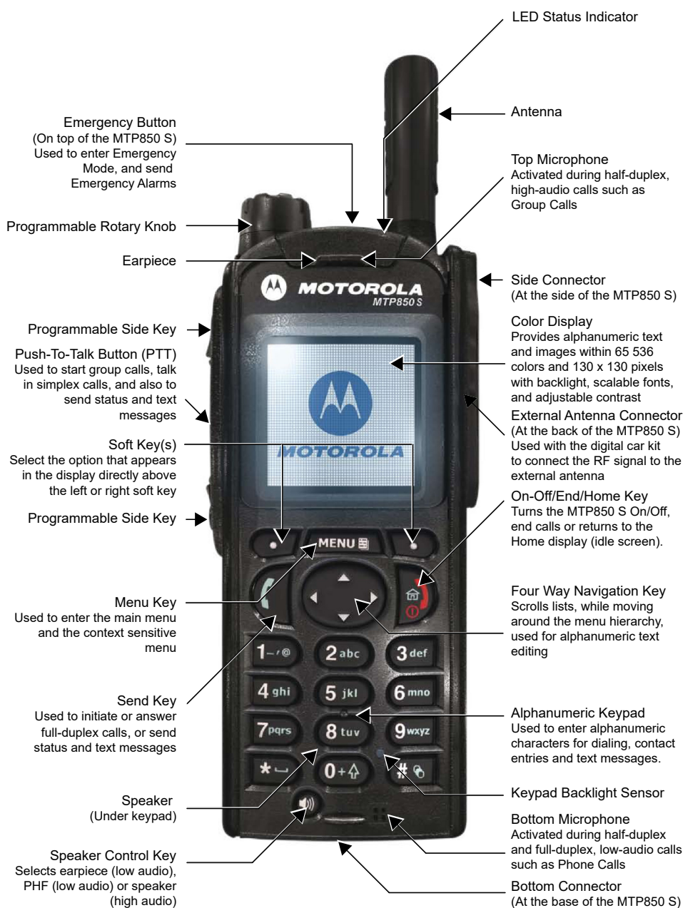
Figure 3-3 MTP850 S/MTP850 FuG Portable Terminal Controls and Indicators
