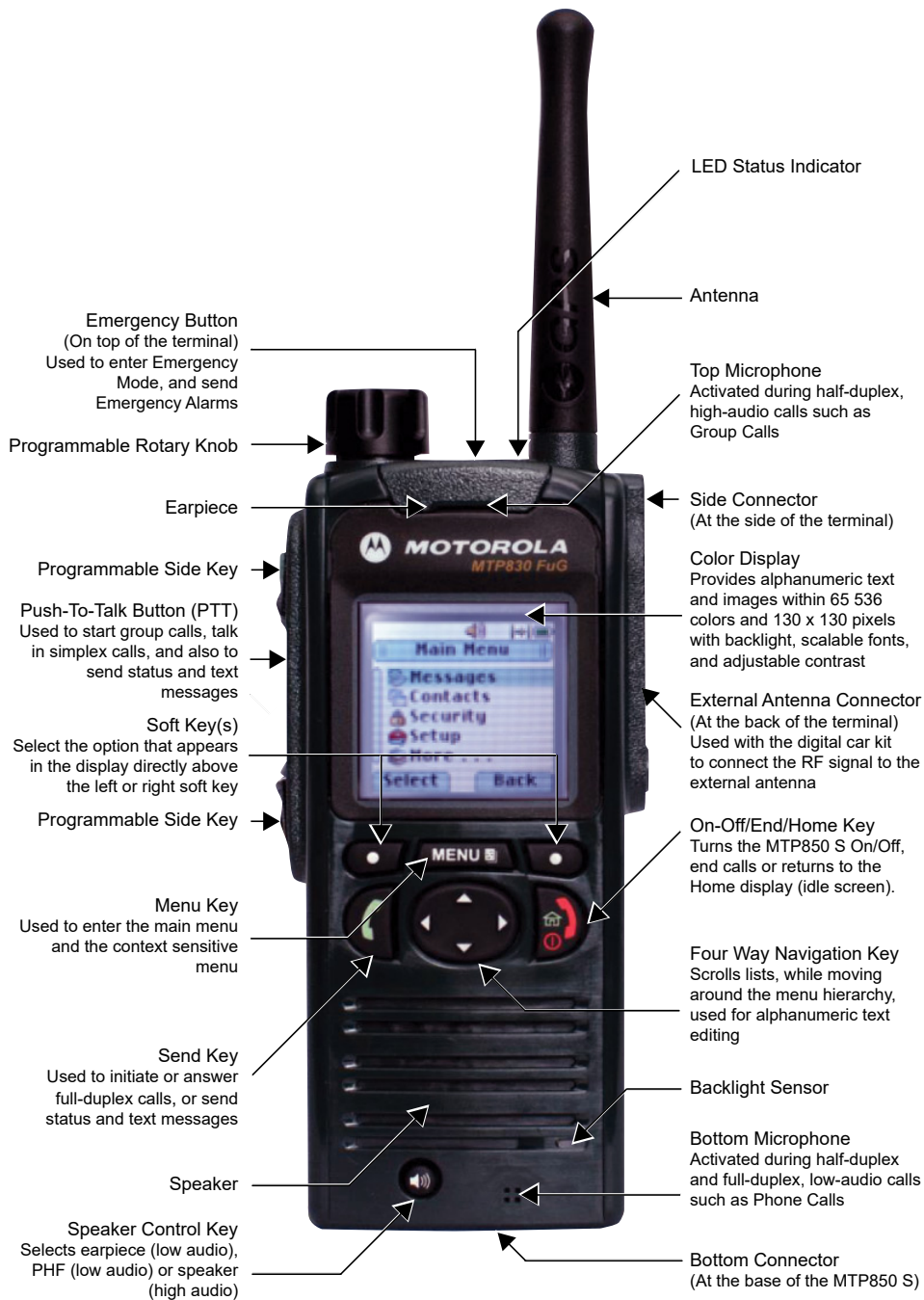
Figure 3-4 MTP830 S/MTP830 FuG Portable Terminal Controls and Indicators
