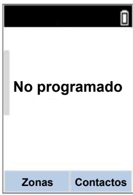
The image shows a radio screen with a black header bar containing a signal strength icon. Below the header, the text "No programado" is centered. At the bottom, there is a blue footer bar with two tabs: "Zonas" and "Contactos". | <b>LED:</b><br>-<br><br><b>Tono:</b><br>Continuo sin programar | El radio está en el estado no programado.                                   |
