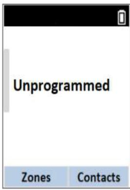
The image shows a white rectangular screen with a black header bar at the top. In the center, the word 'Unprogrammed' is displayed in a large, bold, black font. At the bottom, there are two blue buttons labeled 'Zones' and 'Contacts'. | <b>LED:</b><br>-<br><br><b>Tono:</b><br>Continuo sin programar | La radio no se ha programado.                                                       |
