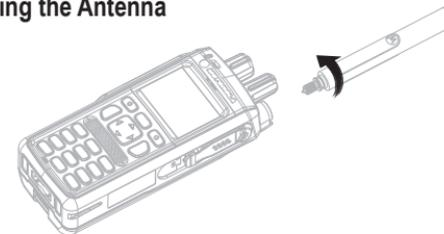
Turn the radio off before attaching the antenna.
