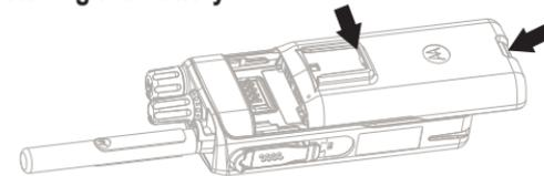
Insert the battery into the compartment.
