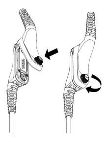
3 To attach the adapter to the radio, hook the Mini GCAI connector and turn the screw clockwise.
