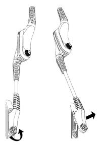
**3** To remove the audio accessory from the adapter, turn the screw anti-clockwise and detach the connector.
