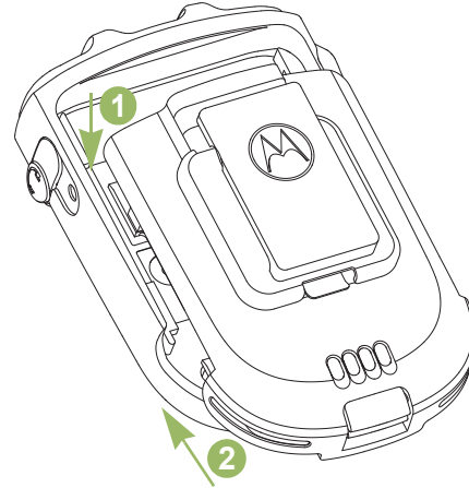
Figure 2.2: Attaching the battery into the WRSM
