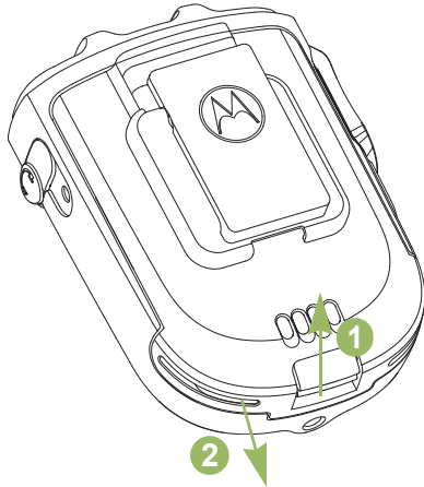
Figure 2.3: Removing the battery from the WRSM
