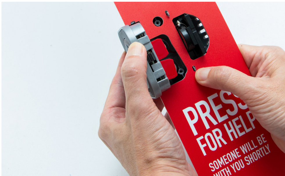
Figure 10: Inserting Bottom Hook
