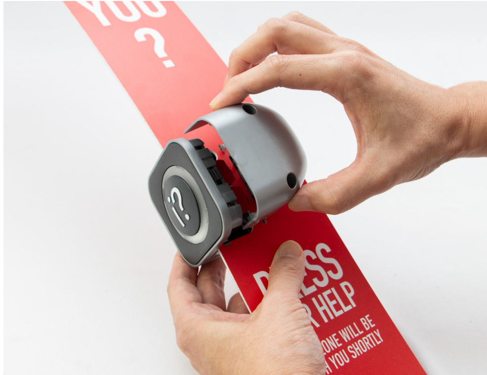
Figure 11: Inserting the Call Button Cover
