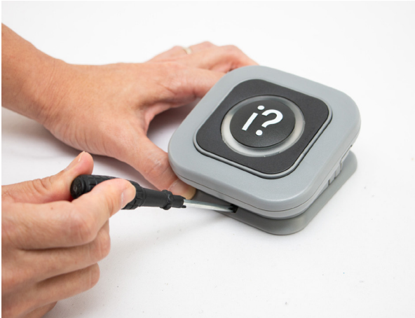
Figure 25: Disassemble the Mounting Plate from the Call Button Base
