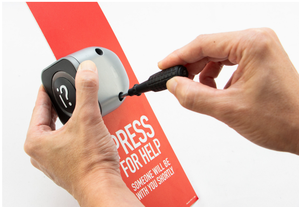
Figure 12: Fastening the Screws
