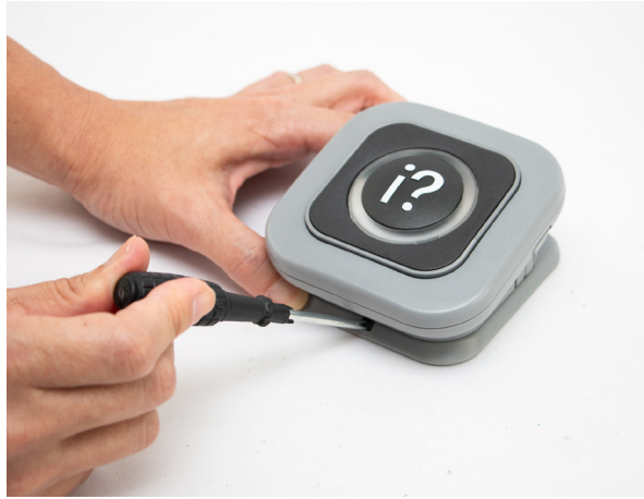
Figure 21: Disassemble the Mounting Plate from the Call Button Base
