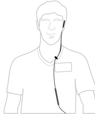
2. Rotate the audio jack connector 90 degrees upwards to lock.
